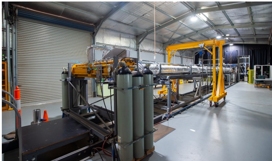
Fig 1. TUSQ hypersonic wind tunnel at the University of Southern Queensland.
