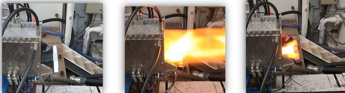
Fig 4. Photos of the test before, during and after the ramjet test
