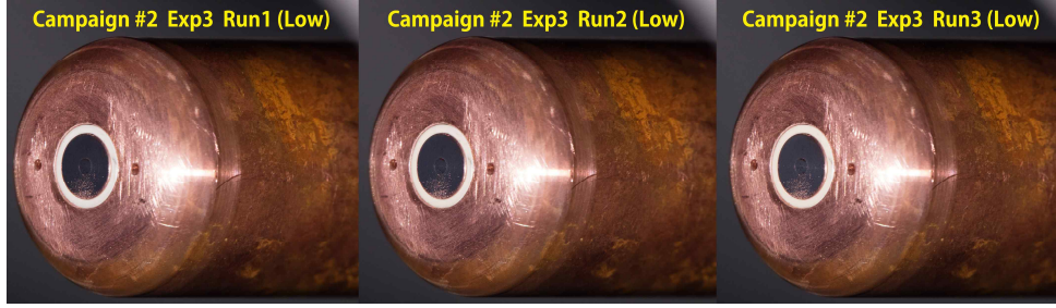
Fig 10. Condition of graphite paste during Exp3 Runs 1–3 (Low Condition)
