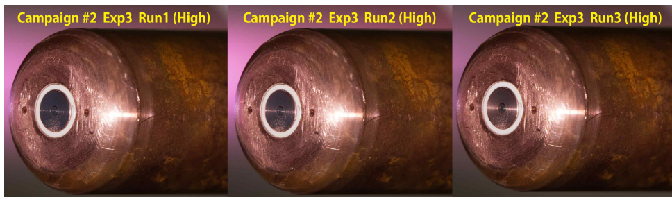
Fig 11. Condition of graphite paste during Exp3 Runs 1–3 (High Condition)
