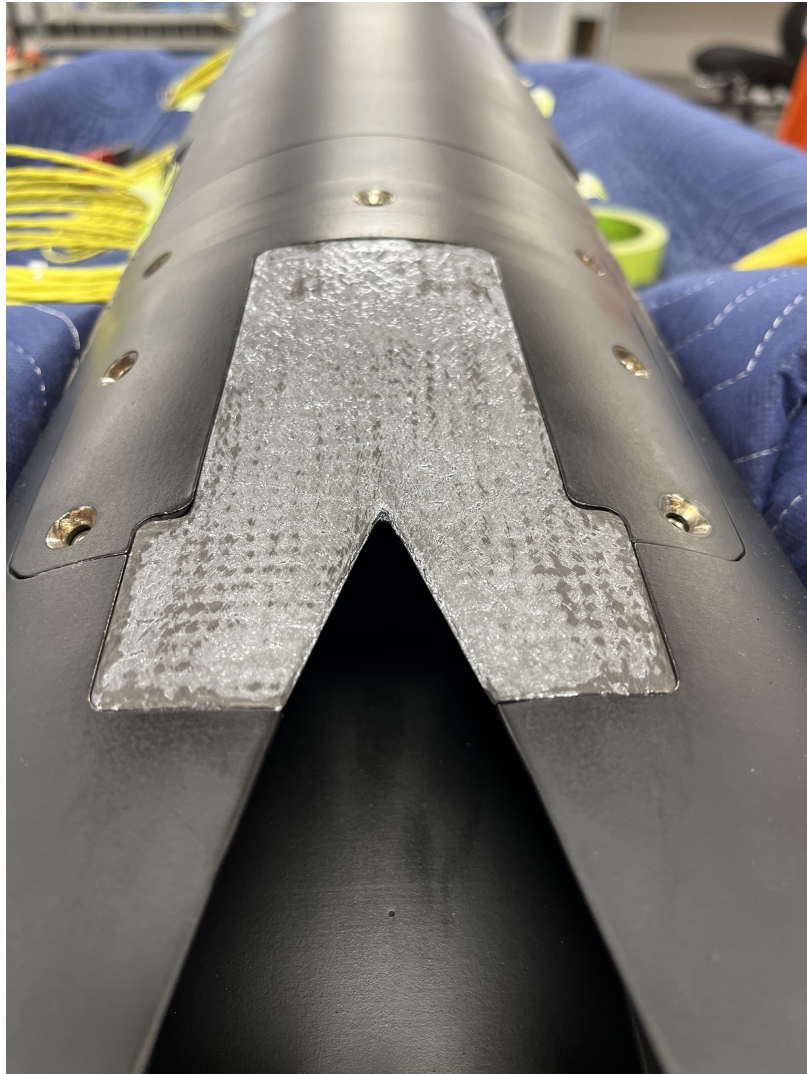
Fig 11. scramjet inlet insert fitted in 3D printed Inconel engine
