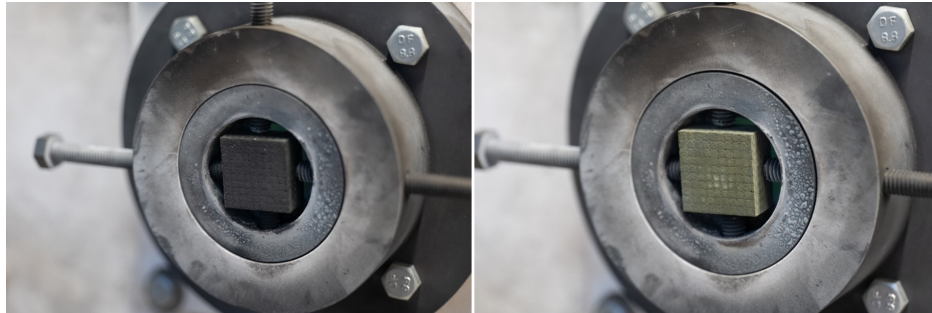
Fig 4. C/SiC specimen before test (left) and after (right)
