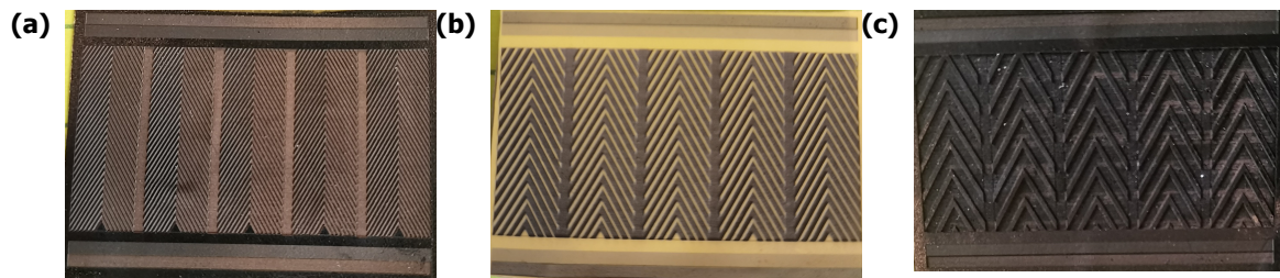
Fig 11. Layout of herringbone riblets with different heights: (a) h = 54 \mu\text{m} , (b) h = 140 \mu\text{m} and (c) h = 215 \mu\text{m} .
