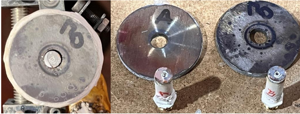
Figure 8. Stainless steel and molybdenum disks and CP20A and CP20B after approximately 30 minutes of cumulative time exposure to plasma jet.
