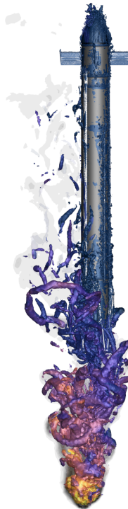
Figure 1. Artistic impression of the CALLISTO vehicle. DES results visualizing the large scale structures using the Q criterion colored by temperature.
