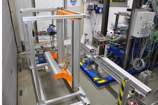
Fig 3. Exhaust Emission Gas Sampling Rig Installed at Test Bench M11.1
