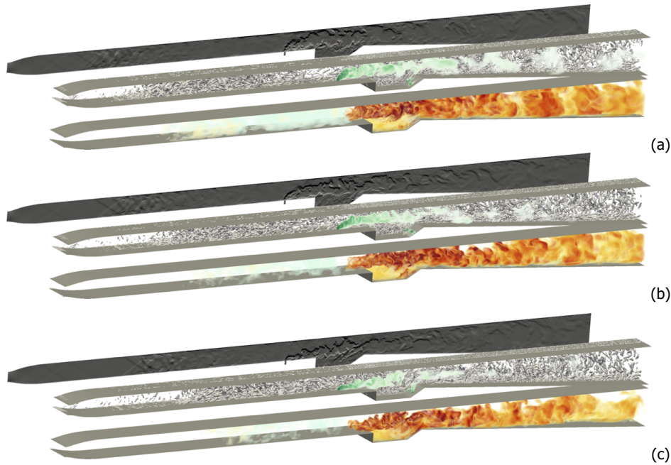
Fig. 4. Perspective views of the flow in terms of the refraction index gradient, \nabla n , the 2 nd invariant of the velocity gradient, \lambda_2 , (gray) and the H 2 mass-fraction (green), and the temperature, T , (warm colors) for (a) Case F1, (b) Case F3 and (c) Case F5.
