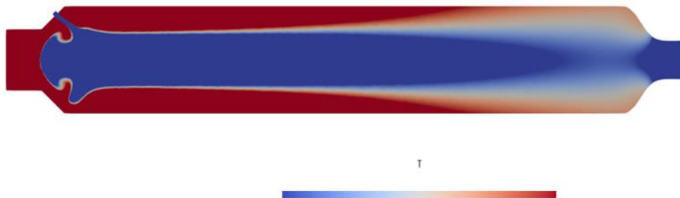
Figure 4 : Example of temperature field inside the mixing chamber
