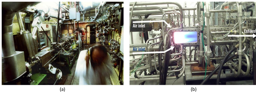
Fig 11. Illustrations of the ONERA test rigs at Palaiseau: (a) the ATD5 test cell dedicated to direct-connected tests in high-Mach flight conditions, (b) test of a typical subsonic combustion ramjet engine in the ATD8 test cell.
