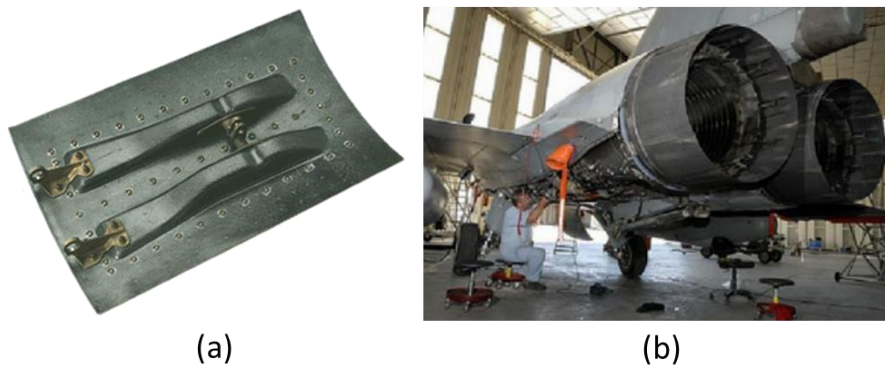
Fig 8. Illustration of a CMC-based exhaust panel (a) of the M88 engine (b).
