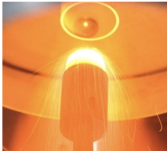
Fig 2. Spallation shown on a FiberForm® sample in the HELMUT facility. Image taken from [17], with permission.
