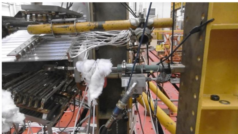
Fig 3. Visualization of interaction between IR lamps heaters and mechanical loads
