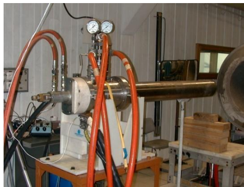
Fig 2: Huels arc heater Illustration
