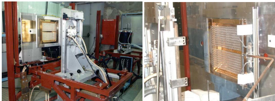
Fig 3: Infra-red flux facility
