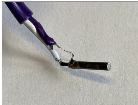
Fig 3. Coaxial thermocouple manufactured in-house with a furnace.
