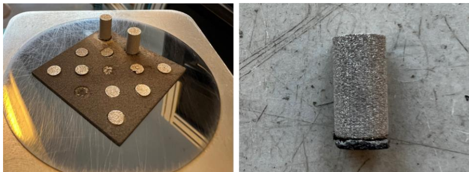
Fig. 6: Ti64 printed on top of a porous printed Si-SiC substrate.
