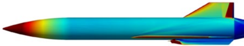
Figure 7: Surface temperature distribution of the HIMICO aircraft (Mach 5)
