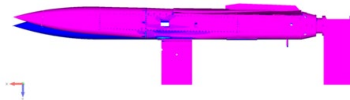
Figure 6: Displacement at wind tunnel starting load
