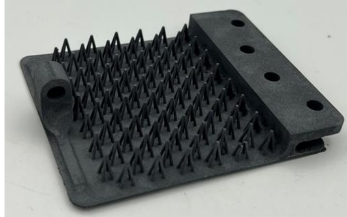
Figure 3: Finished pillar stiffener Si-SiC hot demonstrator component.
