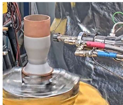
Figure 18: Cold Spray bi-metallic chamber structural jacket with Ni-based alloy [12].
