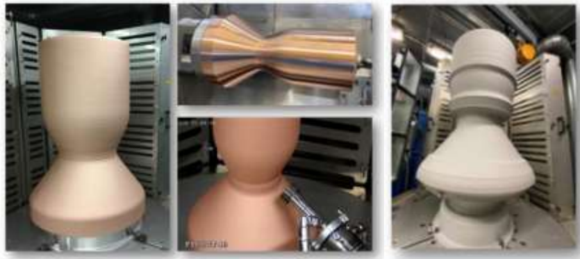
Figure 15: Cold Spray of Cu-alloy – inner liner by ArianeGroup [9].
