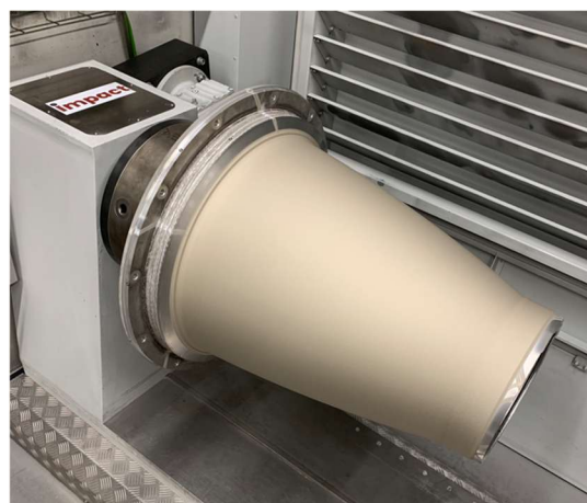
Figure 9: Finished cold sprayed C-103 nozzle extension on Al mandrel [13].
