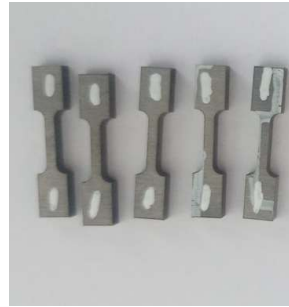
Figure 6: Five tensile specimen with heat Treatment [13].
