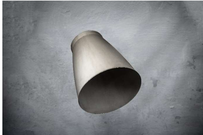
Figure 10: Final C-103 nozzle extension with Al mandrel removed, by chemical dissolution [13].
