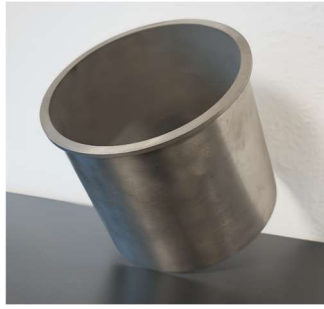
Figure 4: After mandrel removal and post machining [13].
