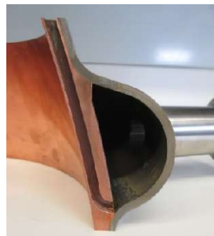
Figure 14: Inner cooling channel structure of manifold [4].
