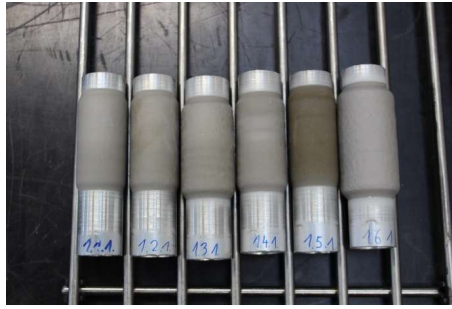
Figure 2: First test tubes to find out basic Cold Spray process parameters and deposition behaviour [13].
