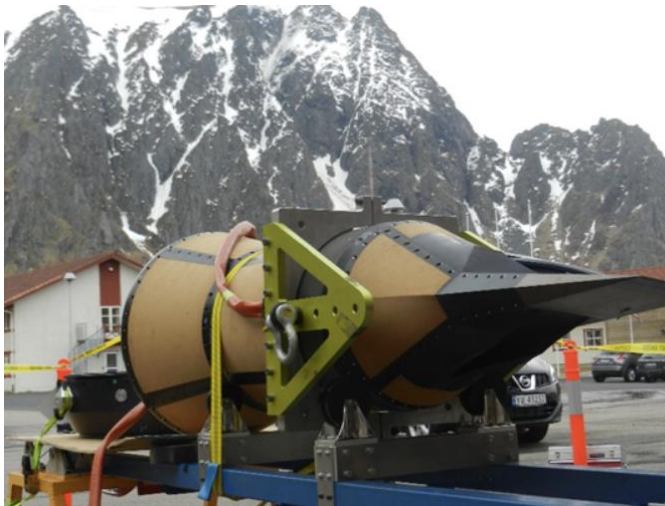
Fig. 34: The HIFiRE-7 free-flyer scramjet payload during rollout (image used with permission from DSTG)
