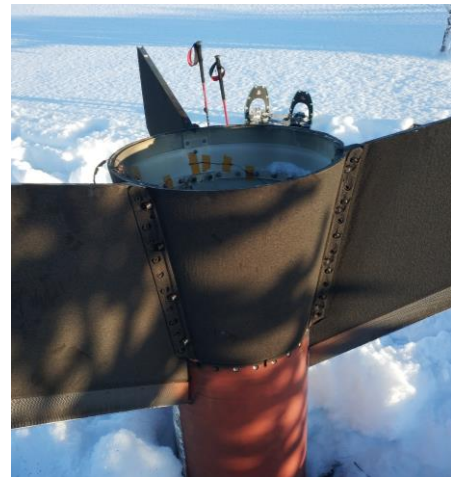
Fig. 15: Charred second stage tailcan assembly post-flight (MAPHEUS-7, 2018)
