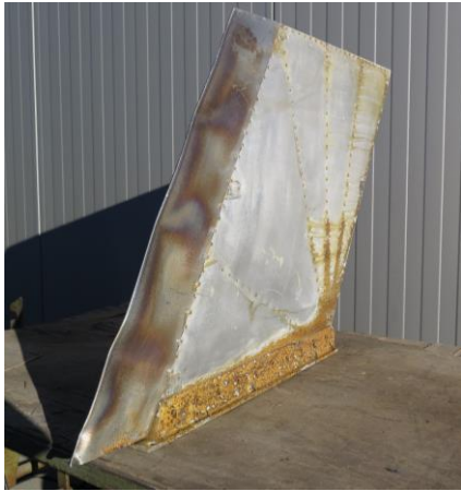
Fig. 11: Heritage FIREX protected S30 fin used on a microgravity Up-and-Over trajectory (TEXUS-48, 2011) after recovery.
