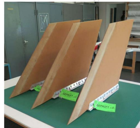
Fig. 12: Cork based thermal protection applied to nosecone and fins
