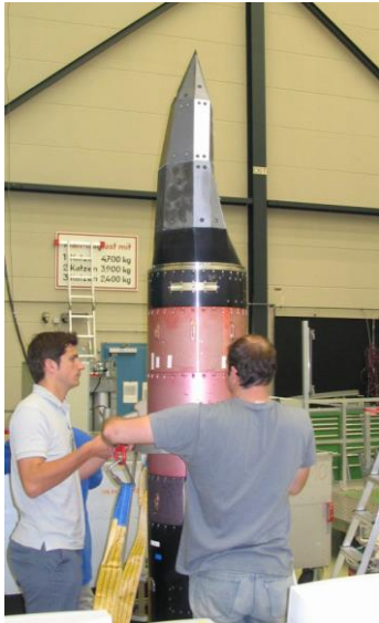
Fig. 24: The asymmetric forebody and payload of SHEFEX-1
