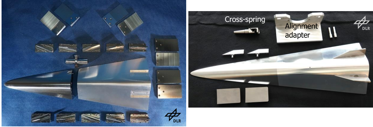
Fig. 6. Components of static (left) and dynamic wind tunnel model (right)
