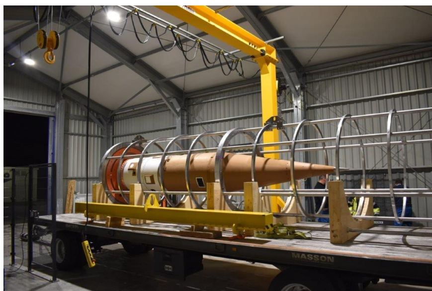
Fig 21 : Upper composite balancing test before final assembly
