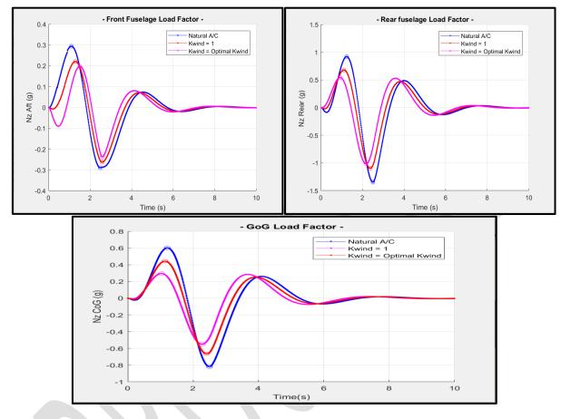
On these figures, we can observe that the optimal elevator order made it possible to significantly reduce the maximum and minimum value of the load factor value compared to the natural aircraft. We nevertheless observe an "**over-shoot**" of the optimal response compared to the natural aircraft around 3(s) for all three sensors along the fuselage.
