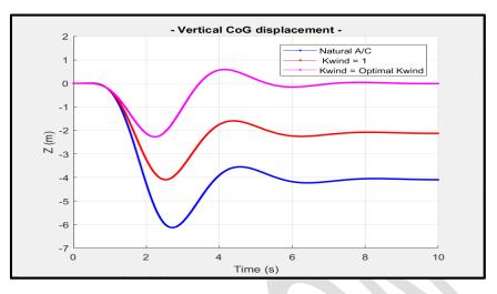
We can observe that, to cancel the gust, the model has a dive movement and that it subsequently repositions itself naturally to its initial position, without the help of any system. This behavior is explained by the zero value of the static gain of the load factor transfer function with respect to wind derivative which by a double integration represents the vertical displacement.
