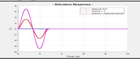
Regarding the optimal elevator order, we can observe that the maximum value is 7 degrees for a load factor reduction of 50(%) at the center of gravity, of 30(%) at the front and 40(%) at the rear fuselage.
