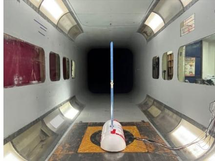
Figure 5: Wing installed in the wind tunnel
