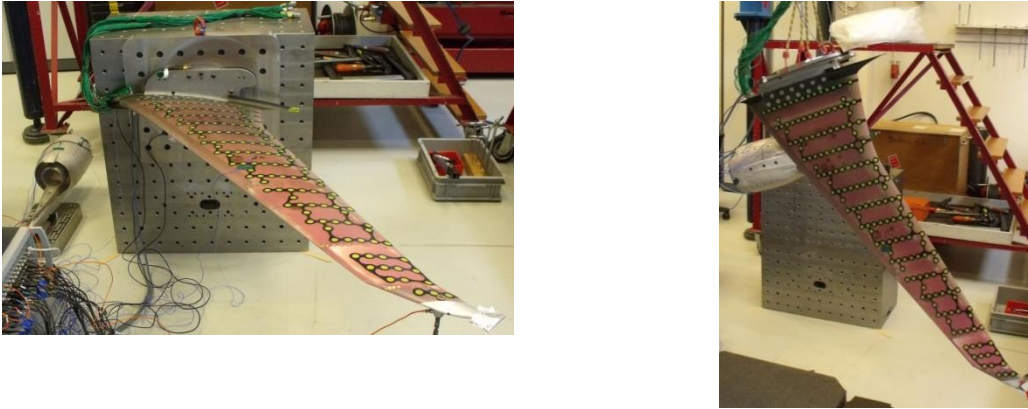
Figure 16: (left) Test set-up for the wing-only in clamped condition and (right) full wing-pylon in free-free condition
