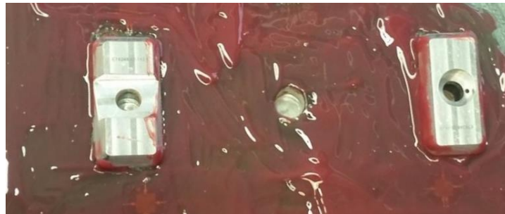
Figure 21: Metal inserts for the pylon to wing connection which have also been covered in adhesive (not shown in the image) during full assembly, resulting in an additional load path
