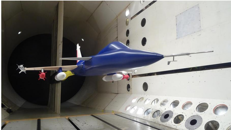
Figure 1: The model installed in the TDT test section.
