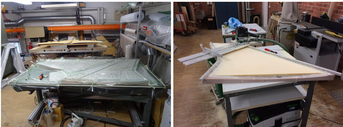
Figure 6: Vacuum bag and milling excess core.
