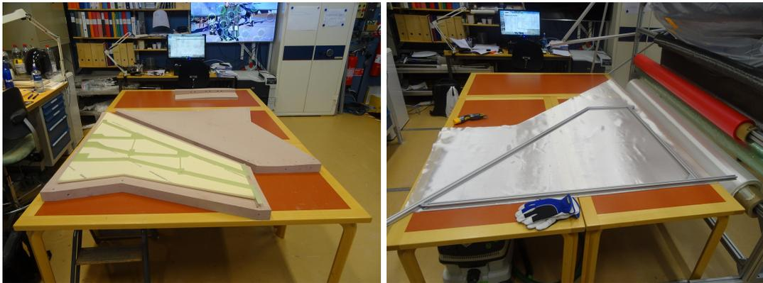
Figure 4: Wing moulds and fiber placement.
