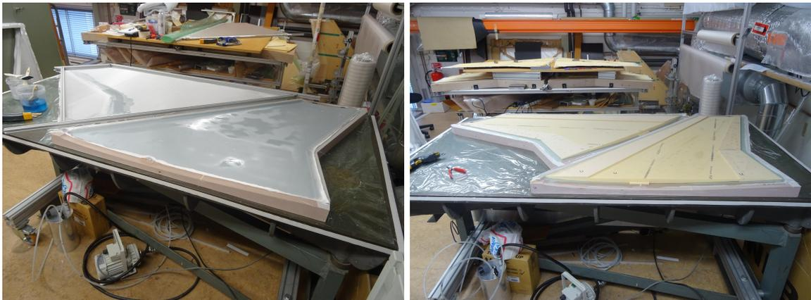
Figure 5: Wetting out and placing core.
