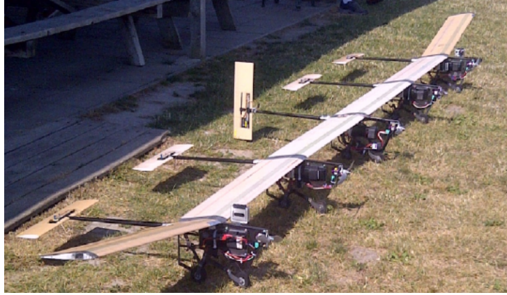
Figure 1: X-HALE aircraft developed in University of Michigan [15]
