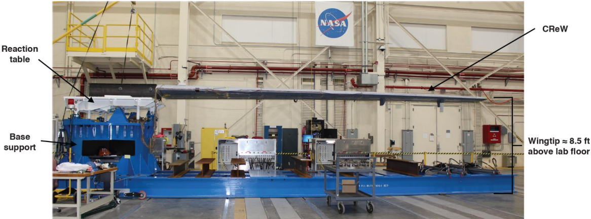
Figure 6: Modal test setup with CRW mounted on the WLTF with wingtip ≈ 8.5 ft above lab floor.
