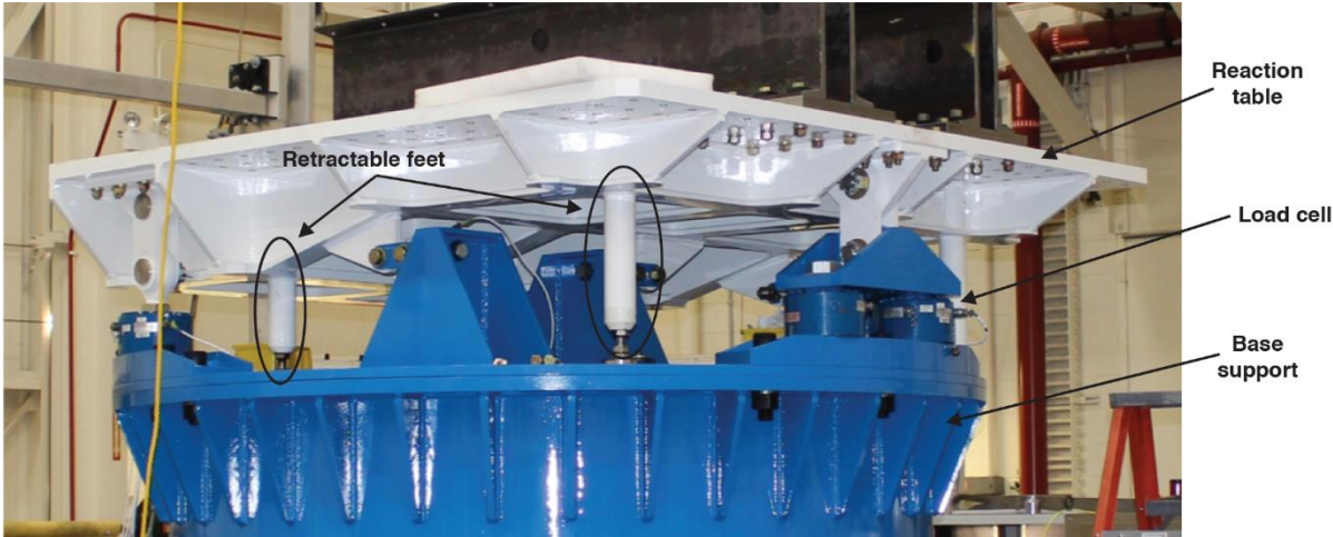
Figure 4: WLTF reaction table supported with 4 retractable feet (2 shown) and 7 load cells (4 shown).
