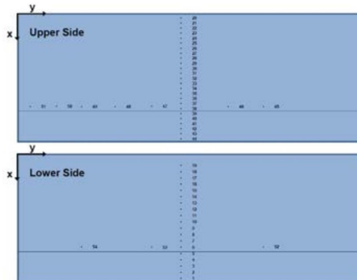
Figure 3: Position of orifices for pressure sensors.
