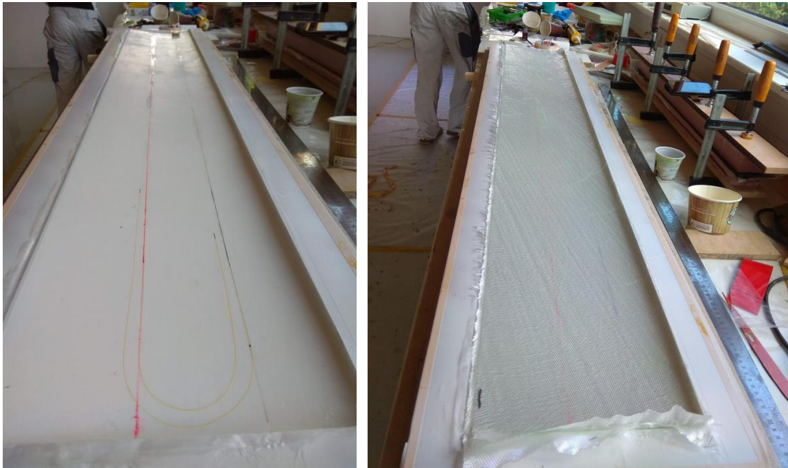
Figure 14: Placement of the strain fiber (left) and a 15° UD glass layer (right)
