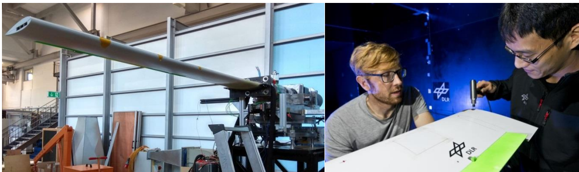
Figure 15: Model mounted on test stand outside the tunnel (left), hammer test inside the tunnel (right).
