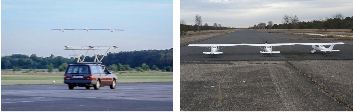
(a) Flight test with an experimental multibody aircraft shortly after lift-off (b) Experimental multibody aircraft for further practical investigations
