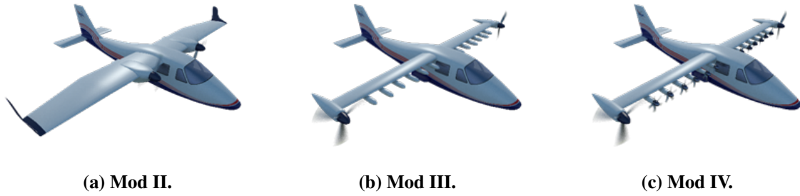
Figure 1: Vehicle configurations of the X-57 project.
