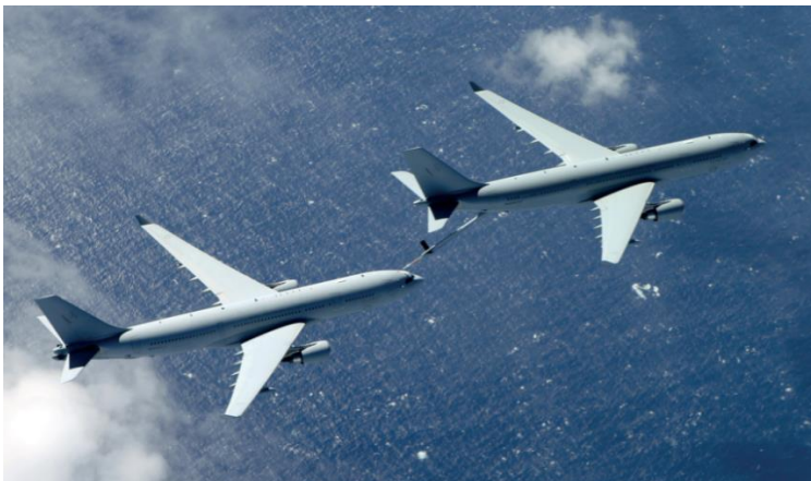
Figure 1 An A330-MRTT tanker aircraft while refuelling to another A330-MRTT acting as receiver.
