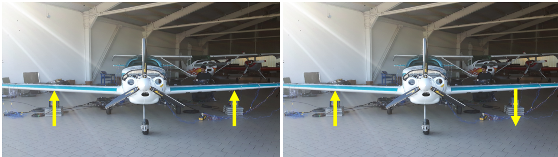
Figure 3: Conventional technique: two sweeps performed by using two shakers in-phase (left) and out-of-phase (right).
