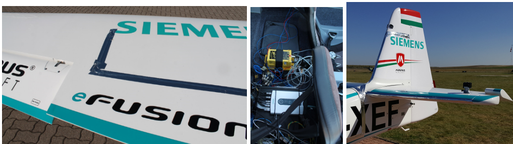
Figure 10: Aircraft instrumentation for flutter testing: accelerometers placed on the left wing (left picture), Simcenter SCADAS XS measurement system in the cockpit (middle) and accelerometer on the vertical tail plane (right picture).
