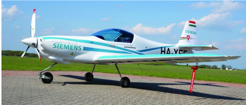
Figure 1: Magnus Fusion aircraft tested with an all-electric propulsion system.
