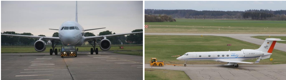
Figure 2: Taxi Vibration Test on the DLR research aircraft ATRA, an A320-200 (left). TVT on HALO on the DLR premises in Oberpfaffenhofen (right).
