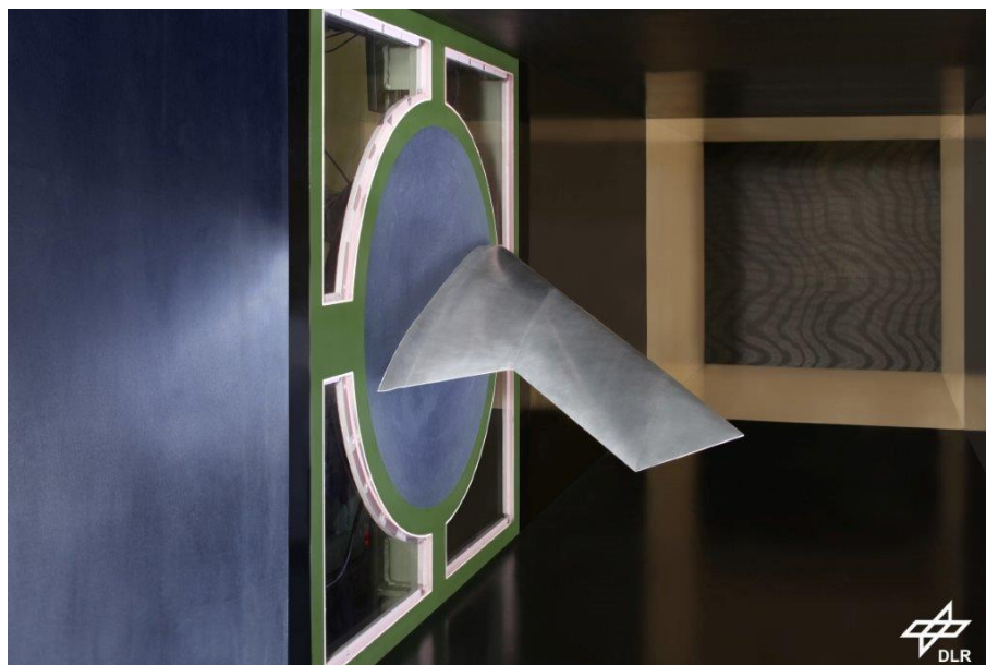
Figure 10: Lambda-wing model of the previous test campaign in the wind tunnel test section.
