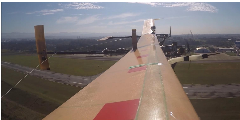
Figure 1: X-HALE aircraft with 4m wingspan that is currently in operation at ITA.
