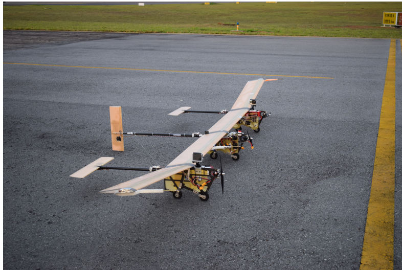
Figure 1: Four-meter-span, vertical-central-tail X-HALE configuration.
