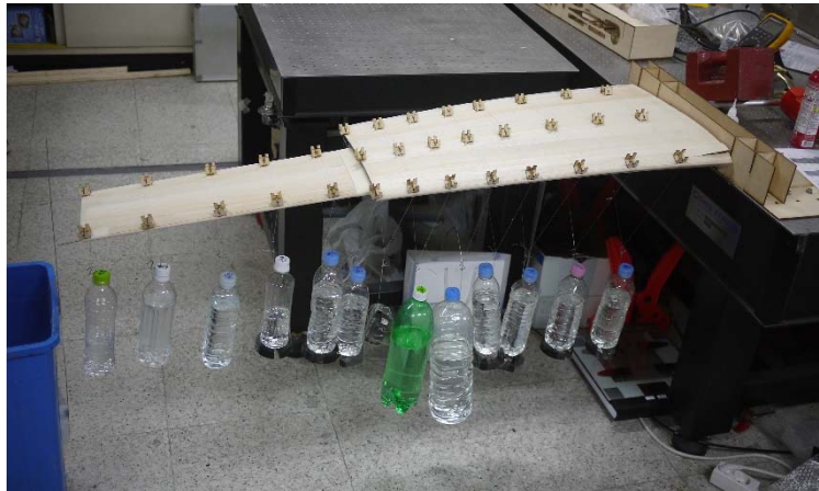
Figure 8: Static test of VSMW.
