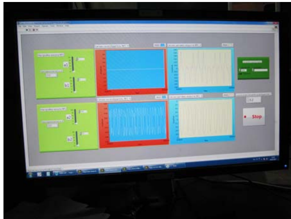
Figure 13: View of the control panel for limit cycle oscillation tests (demonstrator)
