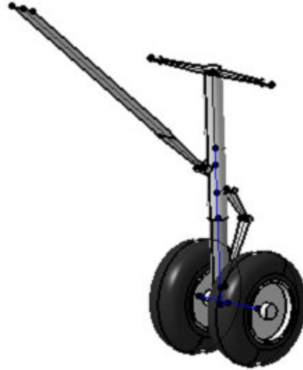
Figure 8. Multi-body model of the nose landing gear.
