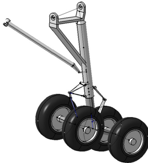
Figure 7. Multi-body model of the left main landing gear.
