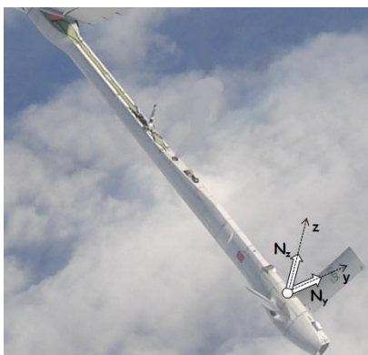
Figure 8 Lateral ( N_y ) and vertical ( N_z ) accelerometers to measure buffeting.
