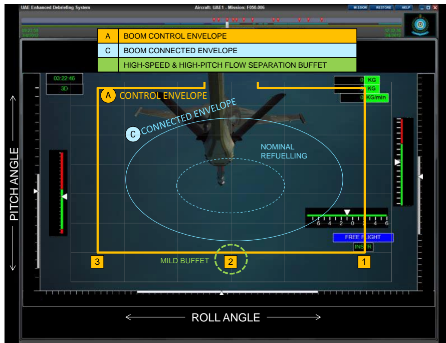
Figure 7 Boom geometrical roll/pitch envelopes: A=Boom control envelope and C=Boom connected envelope. Lower corner of envelope A corresponds to maximum pitch and, at high Mach number conditions, is the zone affected by mild buffet.
