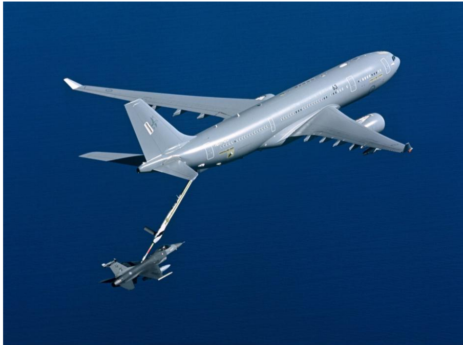
Figure 1 A330-MRTT tanker aircraft dispatching fuel thru the Boom to an F-16.
