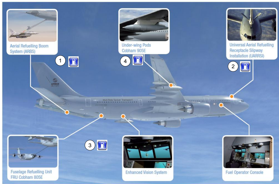
Figure 2: A330-MRTT aircraft with the refuelling devices (under-wing pods and ARBS) and the UARRSI receptacle at the fuselage nose ([1]).
