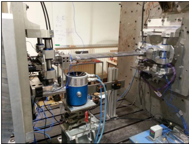
Figure 10: Test set-up for the dynamic qualification
