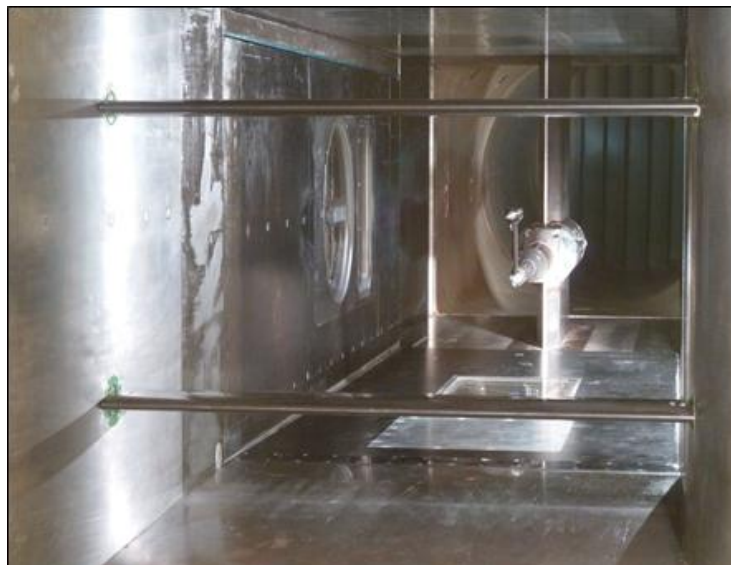
Figure 2: The experimental set-up of the first Wind Tunnel Test: the gust generator (foreground) and the unsteady clinometric probe (background)
