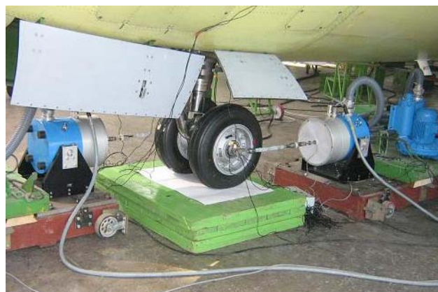
Figure 3: Ground vibration testing of a nose landing gear (NLG) as a part of an airplane. Measurement of tire contact spots during GVT
