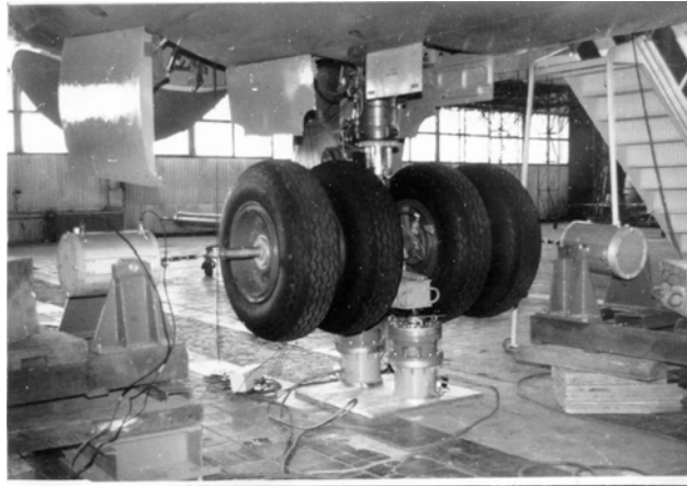
Figure 4: Ground vibration testing of landing gear under compression of strut with the help of air castors
