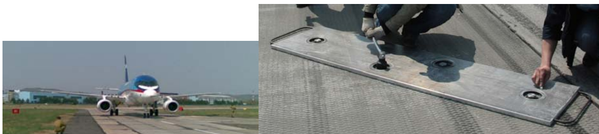
Figure 18: The GT of aircraft with crossing the "shimmy board"
