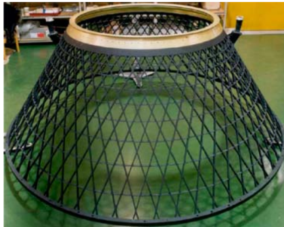
Figure 1: Lattice composite structures in rocket industry (CRISM, Russia)
