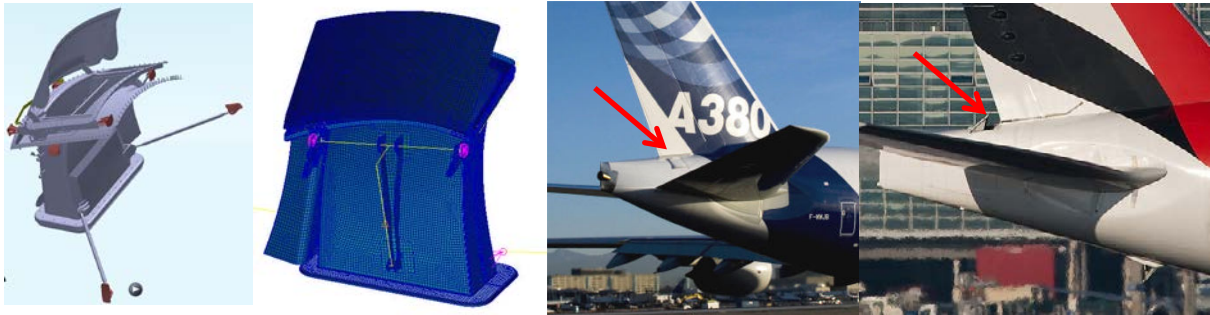
Figure 1: APU air inlet design, FEM and location in the aircraft
