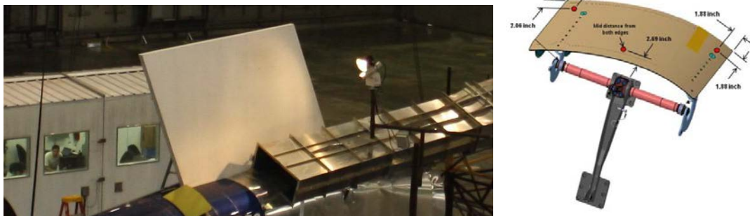
Figure 3: Icing test used for damping calculation
