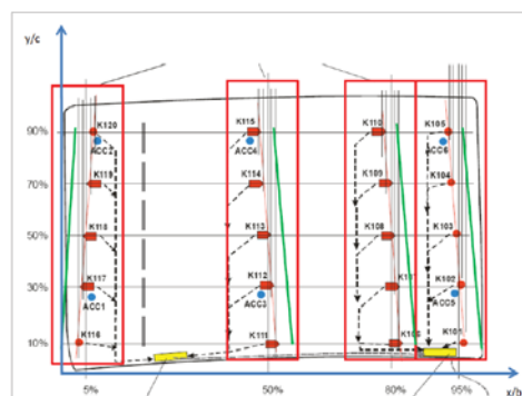
Figure 6: Accelerometer and pressure sensors installed on the WTT.
