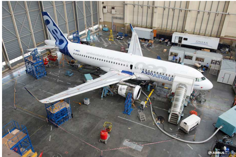
Figure 1: GVT campaign of the A320 NEO PW MSN 6101 in AIRBUS facilities (Toulouse, France)
