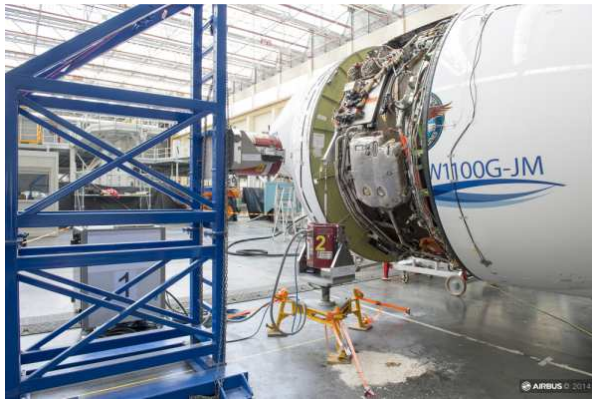
Figure 3: View of the Z excitation of the left-hand side engine
