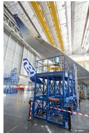
Figure 4: View of the Z excitation of the right-hand side wing
