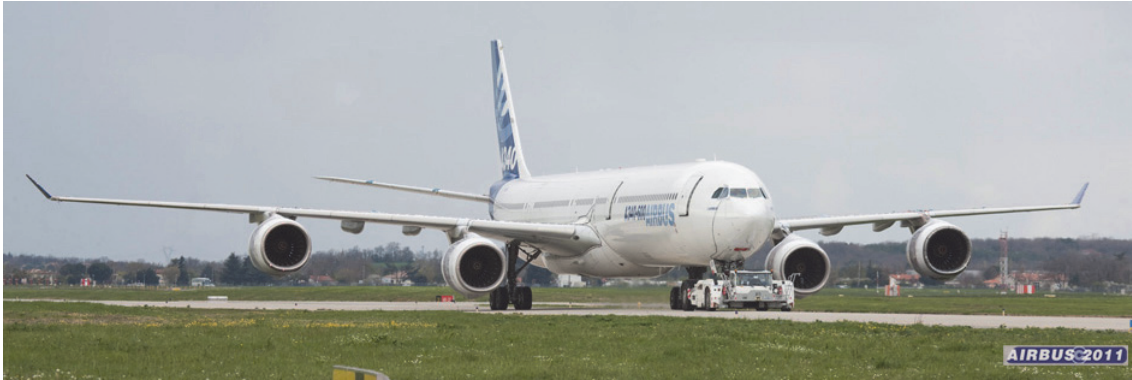
Figure 9: Taxi Vibration Test on an A340-600 long range aircraft at Airbus in Toulouse
