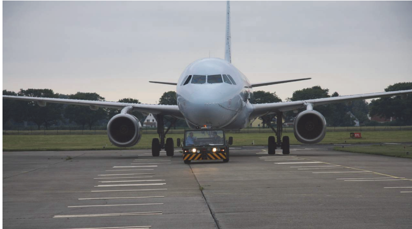
Figure 7: Taxi Vibration Test on the DLR research aircraft ATRA, an A320-200
