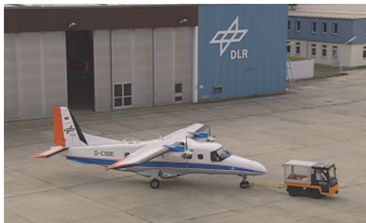
Figure 5: Taxi vibration test on Do228 commuter class aircraft pulled by a tractor in front of the old DLR flight operations hangar in Braunschweig, Germany
