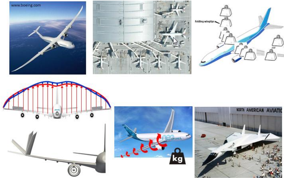
Figure 1: Pictorial explanation of the context and opportunity of folding wing tips for load alleviation.
