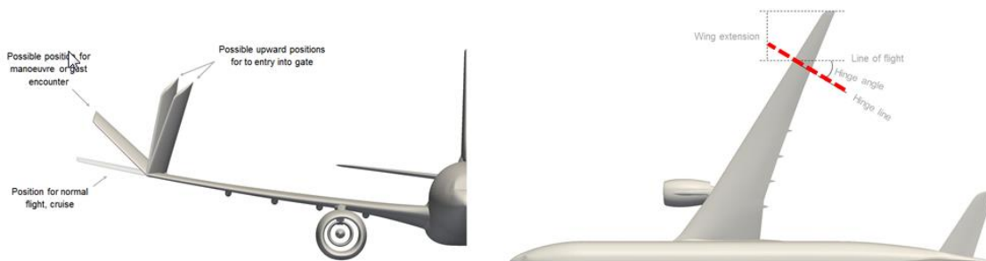
Figure 3: Definition of hinge flare angle (right) and typical wing tip positions at gate and under limit load conditions (left)
