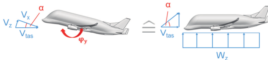
Figure 3: Similarity of pitch mode and vertical gust/heave velocity for frequency zero
